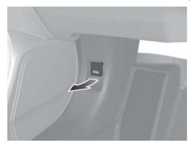
2. Locate the hood latch lever, pull the lever, and lift the hood.
